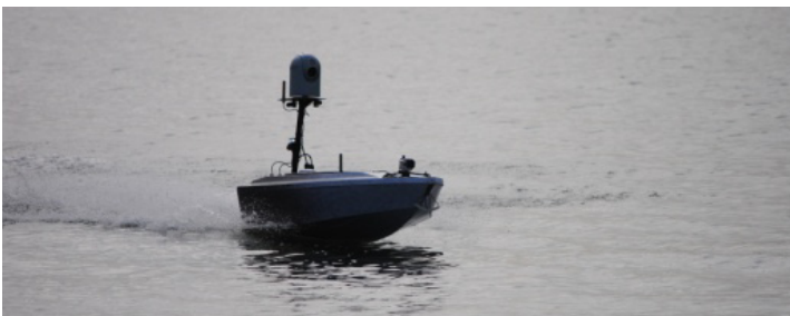
Command and Control (C2) interface for Riverscout USV, an advanced unmanned boat that carries a pan/tilt/zoom camera gimbal for remote inspection, reconnaissance and surveillance along rivers and estuaries.
